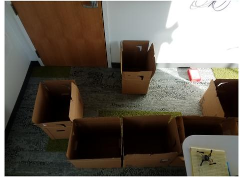
Figure 2: Environment setup for mapping. The middle box is removed during the initial mapping and replaced for obstacle avoidance.
